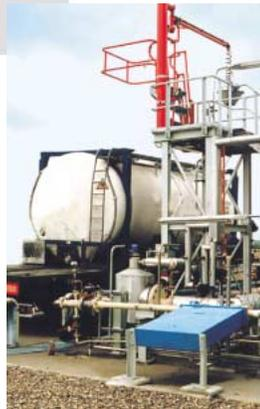
The flexibility of the Rheonik range in terms of applicability and accuracy is due to the patented mechanical arrangement of each meter. Each flowmeter has two measuring tubes parallel to one another and formed into the unique Omega shape, oscillating in opposing directions.
